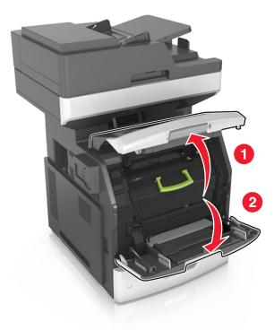
Pull out the toner cartridge from the printer using the handle.
